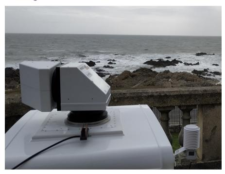
having a lidar [in your project] opens a lot of doors for full-scale experiments. It is the best instrument to measure the atmospheric flow in the wind farm environment by providing space resolution."
